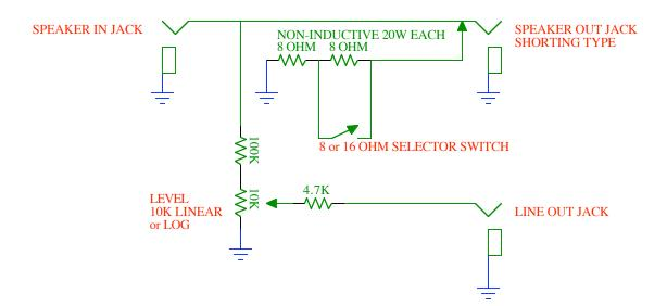
When not using a speaker the non-inductive resistive load is switched in and can be set for 8 or 16 ohm amp outputs. The Non-Inductive resistors are RS Cat#271-120
